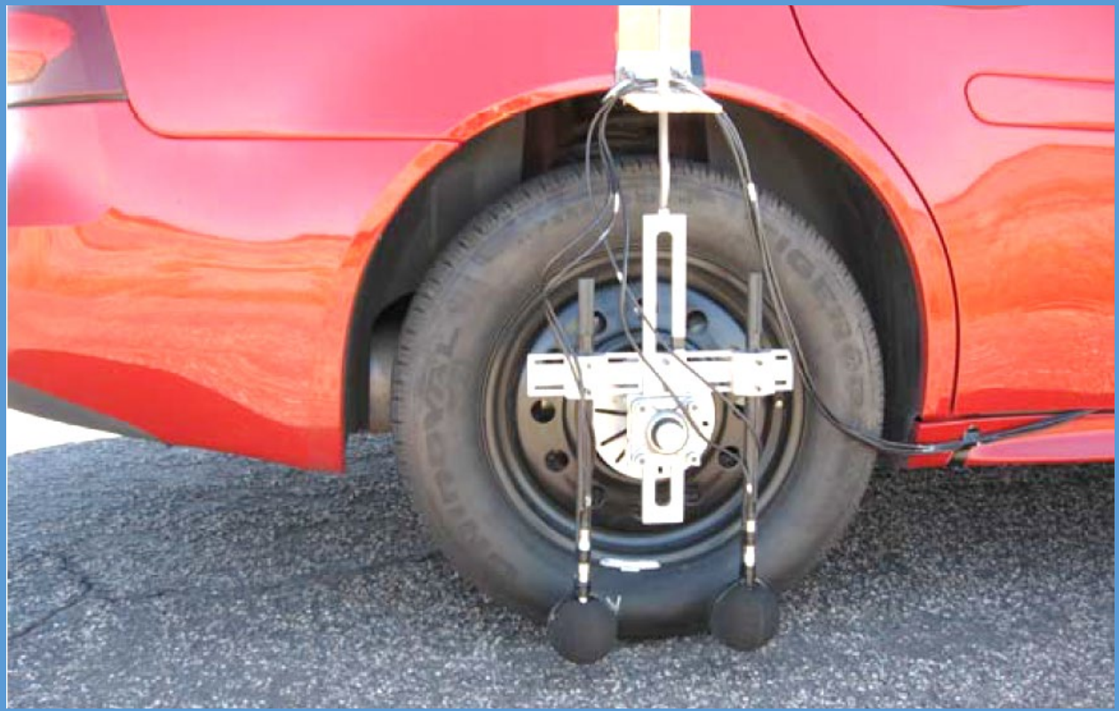
4 Figure 1. Top: GIS Webserver showing 24-mile-long Santa Clara County Route 85 (SCI- 5 85) corridor in Silicon Valley with extensive sound wall system shown in red. Bottom: 6 AASHTO Standard T-360 On-Board Sound Intensity (OBSI) measurement probes used to 7 map pavement acoustics.
